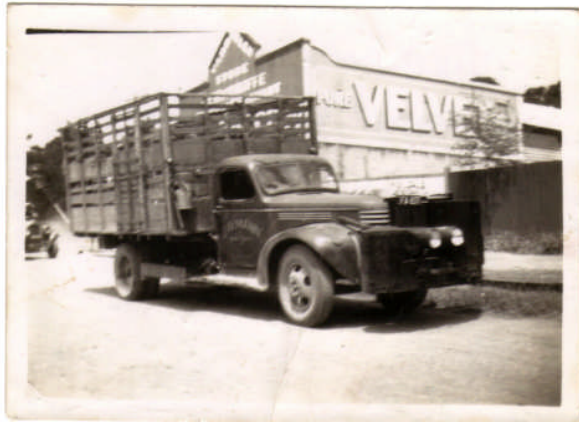
Jack Mann's cattle truck c.1941 with a gas producer on the front
